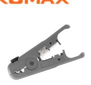
The NMC-S501B tool is designed for stripping and trimming twisted pair, coaxial and flat multicore cables. The tool is equipped with 2 guiding sockets for cleaning round cables (with an outside diameter of up to 9.5 mm), two knives with limiters for stripping flat cables. There is also a knife for cutting cables.
