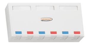
Surface mount box are an integral part of the horizontal subsystems of SCS and are intended for connection of terminal equipment in workplaces. Structurally, the sockets can be made in two versions: as a complete solution with soldered RJ45 ports and IDC connectors and in the form of a plastic casing into which Keystone plug-in modules are separately installed.
