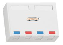
Surface mount box are an integral part of the horizontal subsystems of SCS and are intended for connection of terminal equipment in workplaces. Structurally, the sockets can be made in two versions: as a complete solution with soldered RJ45 ports and IDC connectors and in the form of a plastic casing into which Keystone plug-in modules are separately installed.
