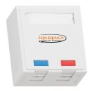
Surface mount box are an integral part of the horizontal subsystems of SCS and are intended for connection of terminal equipment in workplaces. Structurally, the sockets can be made in two versions: as a complete solution with soldered RJ45 ports and IDC connectors and in the form of a plastic casing into which Keystone plug-in modules are separately installed.
