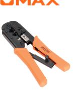
Crimping tools (**Crimper**) are designed for crimping Registered Jack (**RJ**) type connectors on telephone cables and data transmission. **NMC-568R** is designed for crimping RJ45 / 8P8C, RJ12 / 6P6C and RJ11 / 6P4C type connectors. The tool is also equipped with a device for stripping and cutting cables.
