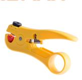
Tool NMC-350 is designed to remove the insulation and trimming with twisted pair. The presence of the wheel for fine adjustment of the depth of the knife moves allows you to make an accurate cut without damaging the insulation of the conductors under the outer shell. A distinctive feature of the NMC-350 is the presence of a spring-loaded cradle for a smooth and uniform course when scrolling around the cable. And the ergonomic design will provide even greater comfort when working.
