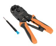
Crimp tools (crimpers) are designed to crimp connectors of the Registered Jack (RJ) type on telephone cables and data cables. NIKOMAX NMC-2008AR is designed for crimping RJ45 / 8P8C, RJ12 / 6P6C, RJ11 / 6P4C, 4P4C and 4P2C connectors. The tool is equipped with a device for stripping and trimming the cable. This tool is professional, thanks to the "end" crimping feature and multi-functionality.
