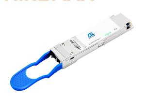
Compliant with QSFP+ SFF-8436 MSA for mechanical, low speed electrical and 2-wire serial management interface for control and real-time monitoring. Supports 40 Gbps data rates links from 2m to 10KM over a standard SMF QSFP+ footprint (Quad Small Form-factor Pluggable) with 2 unidirectional LC SMF optical connector receptacles 38 pin hot pluggable edge connector electrical interface based on QSFP+ MSA.
